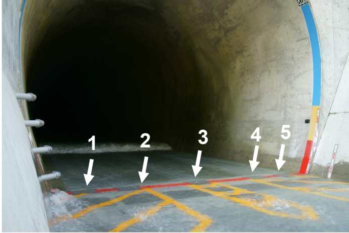
Figure 4. The Koshi Dam SBT outlet with five IPs installed. White arrows show the impact plates.
