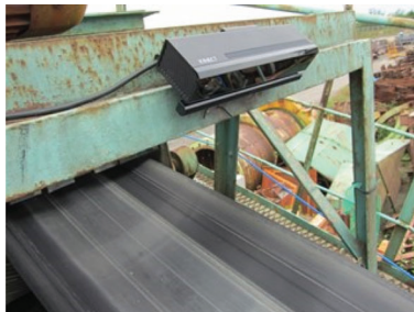
Figure 8. 3D laser scanner above the belt conveyor
