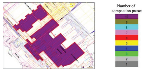
Figure 5. Screen for controlling the number of vibrating roller compaction passes
