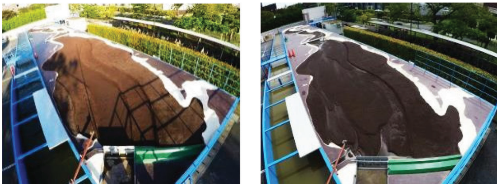
Figure 12. Riverbed before and after the flood (Case-2)
