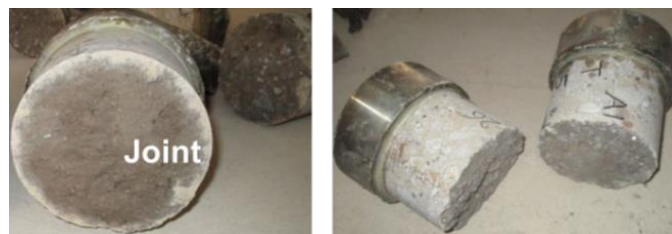
Figure 9. Photograph after Direct Tensile Strength Test of Warm Joint Treatment
