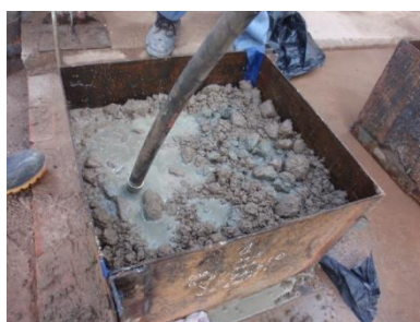
Compacting GE-RCC (Method 2)
