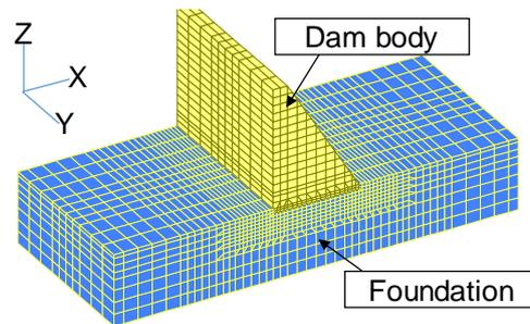
Figure 5. The model for 3D FEM analysis
