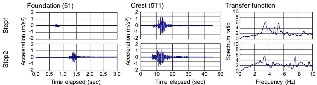
**Figure 4. Acceleration waveforms and response spectrum ratios along X**
