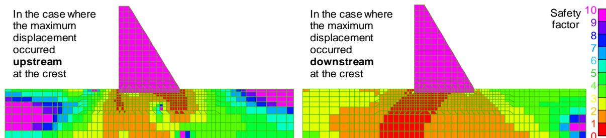
Figure 10. The distributions of local shear safety factors in step 2
