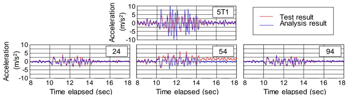
**Figure 8. The typical acceleration waveforms along X at typical points in step 2**
