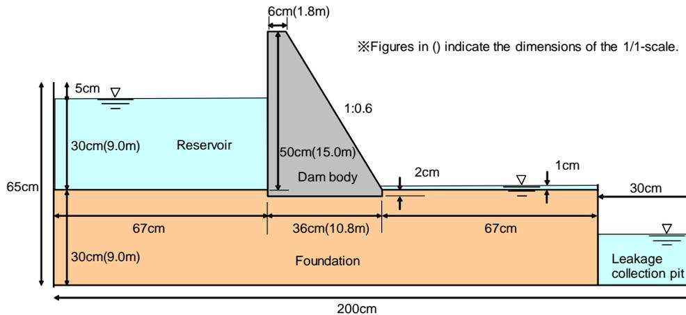
**Figure 1. The dimensions of the 1/30-scale model**
