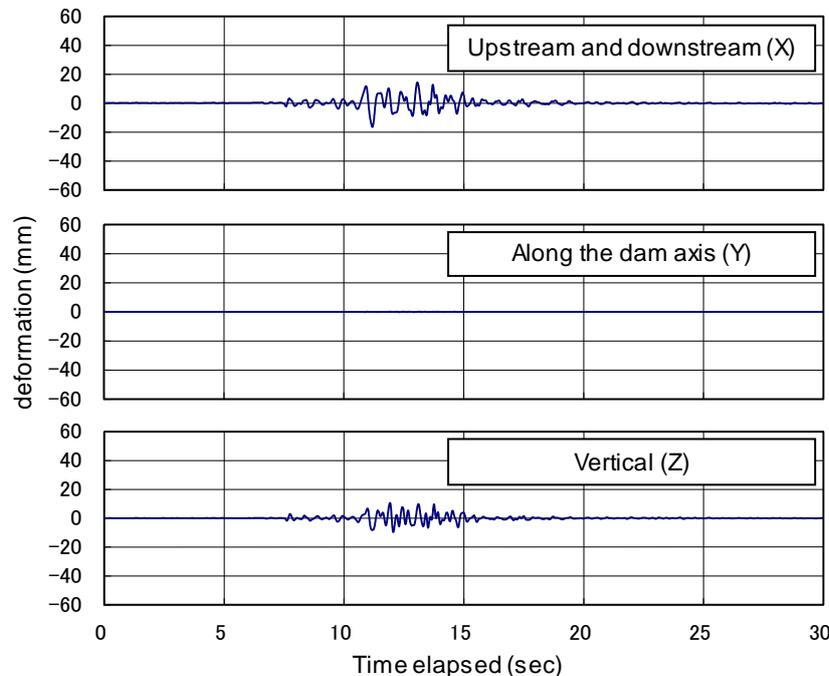
Figure 9. Displacements at typical position (54) in the dynamic analysis
