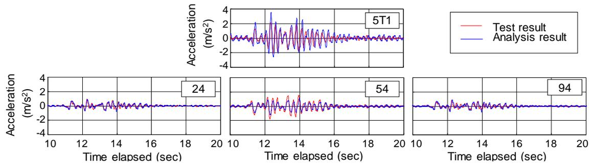
**Figure 7. The acceleration waveforms along X at typical points in step 1**
