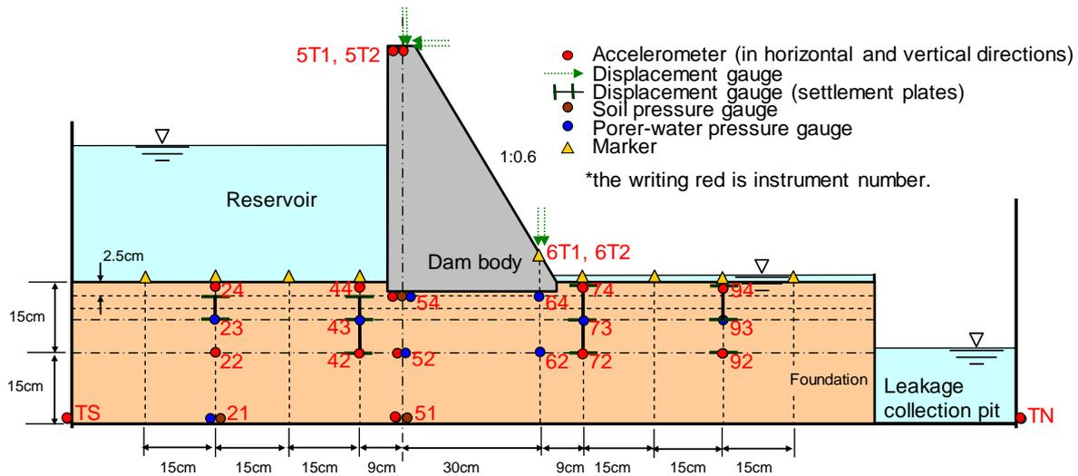
Figure 2. The allocation of measuring instruments
