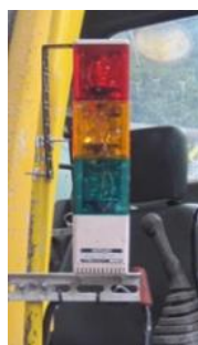
Figure 16. Indication of the state of compaction using revolving light
