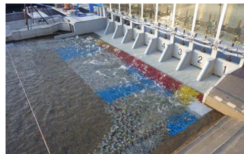
Figure 7. Fully 3D hydraulic scale model
