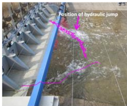
Figure 12. Flow regime of semi uniform opening gate operation
