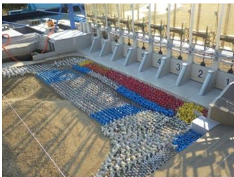
Figure 20. Stability of maintenance plan after design flood 11,130m 3 /s
