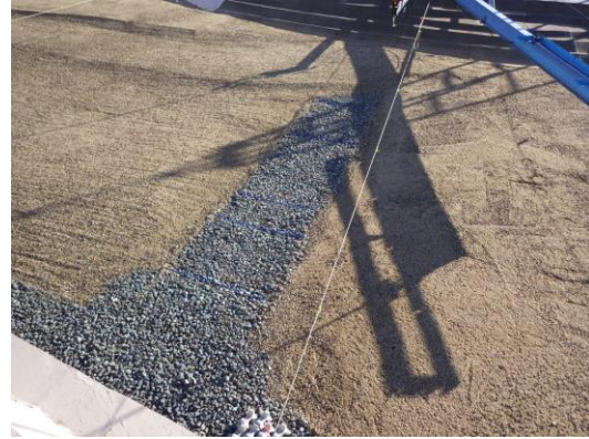
Figure 6. Protection work against riverbed lowering by hydraulic scale model experiment
