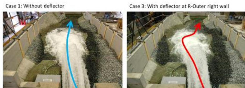
Figure 8. Difference in Diving Points between the Cases with and without a Deflector
