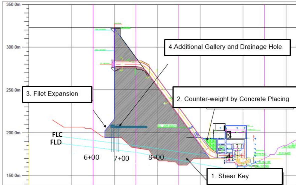
Figure 7. Outline of Wedge Analysis Model and Measures for Stability
