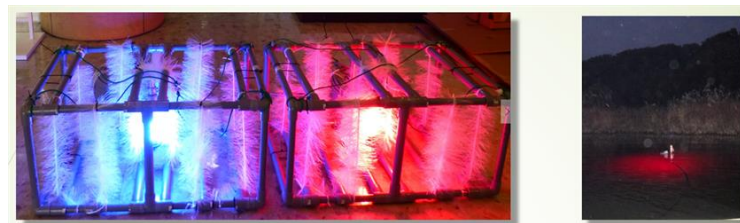
Figure 9. Field verification testing equipment for LED Radiation efficacy and its operating status at the experimental pond
