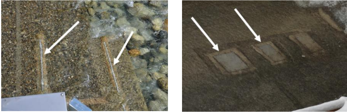
Figure 2. a) Hydrophones installed at Yodagiri River, b) Geophones installed at Ashiarai dani, Hodaka Observatory, DPRI, Kyoto University in Japan
