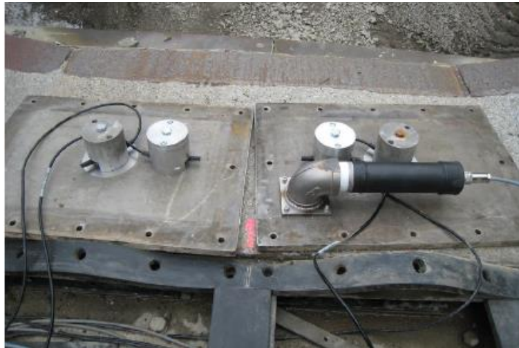
Figure 4. The inside of geophone (left) and plate microphone and vibration sensor (right)
