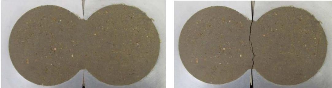
**Figure 10.** Specimen before (left) and after (right) the direct tensile test
