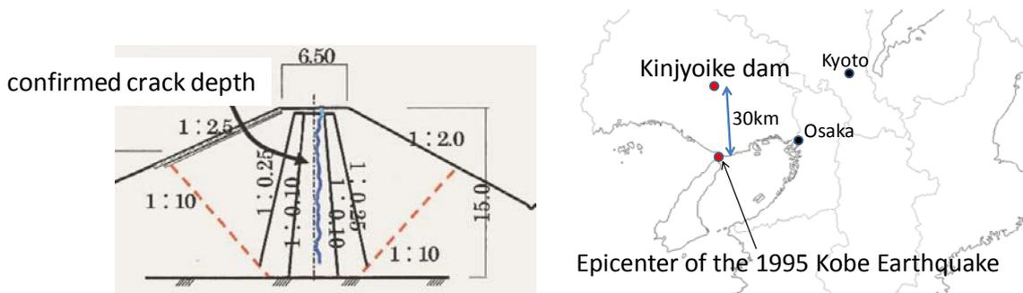
**Figure 3.** Crack depth of the Kinjoike dam after the Kobe earthquake in 1995 (left) and location of the Kinjoike dam (Hyogo Prefecture, 1996)
