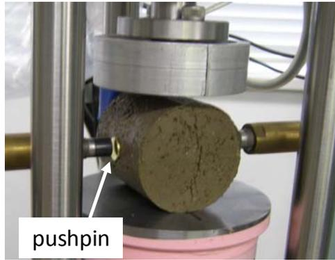
**Figure 6.** Photo of the splitting tensile test
