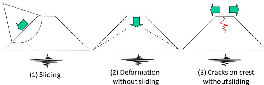
**Figure 1.** Typical damage types of embankment dams due to recent large earthquakes
