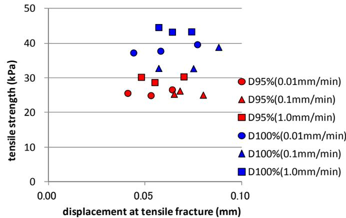
Figure 13. Relationships between displacement at failure and tensile strength
