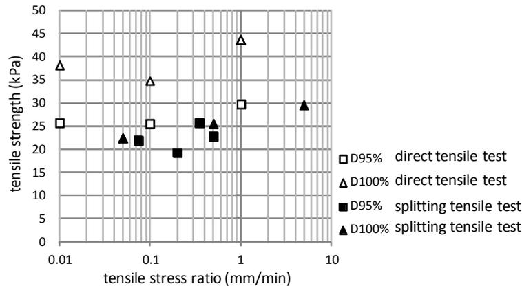
Figure 14. Comparison of results of splitting and direct tensile tests
