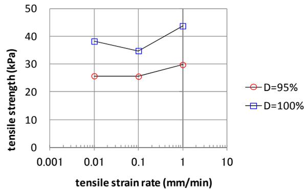
**Figure 12.** Relationships between tensile strain ratio and tensile strength
