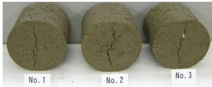
**Figure 8.** Specimens after the splitting tensile tests (D=100%)
