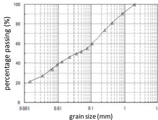
**Figure 5.** Grain size distribution of test material
