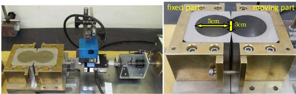
**Figure 9.** The direct tensile test equipment (left) and the test mold (right)
