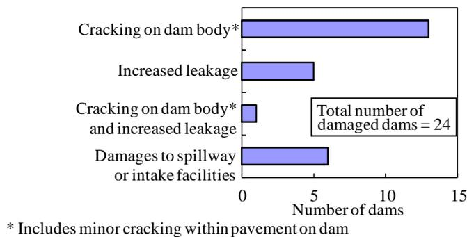
**Figure 4.** Damage types of embankment dams after the Tohoku earthquake in 2011 (Yamaguchi et al., 2012)
