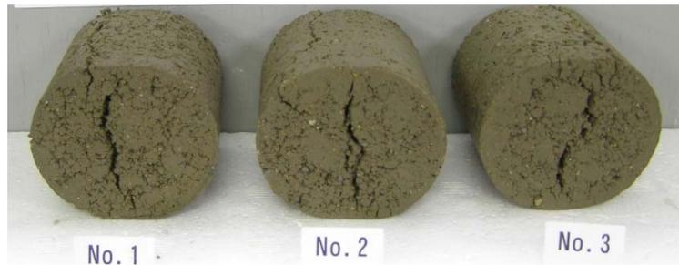
**Figure 7.** Specimens after the splitting tensile tests (D=95%)
