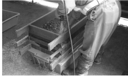
Figure 6. Implementation status of simple test method with water rinse at Tobetsu Dam
