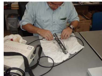
Photo 3. Measurement of ultrasonic wave propagation velocity
