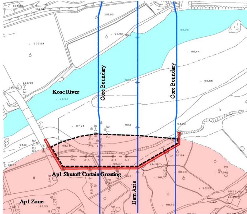
Figure 8. Ap1 Shutoff Curtain Grouting Plan
