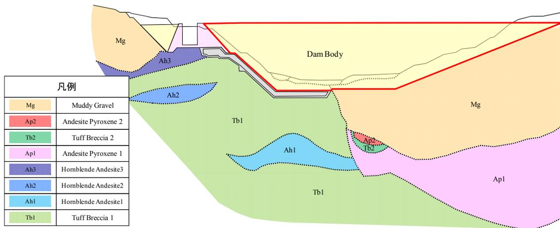
Figure 2. Cross-section under the Dam
