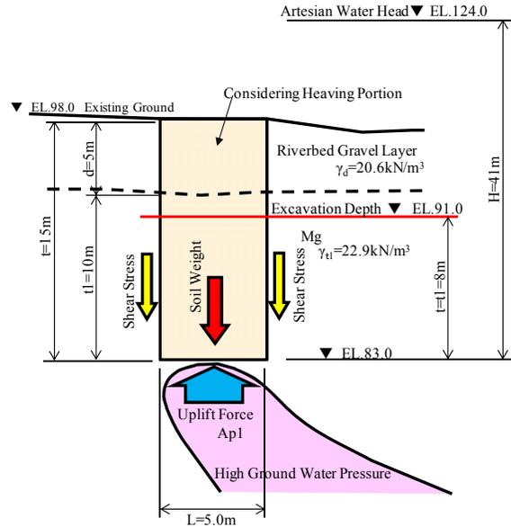
Figure 6. Heaving Model by Artesian Water Head
