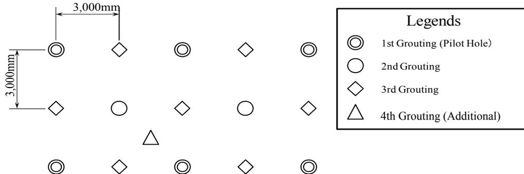
Figure 12. Ap1 Treating Blanket Grouting Layout
