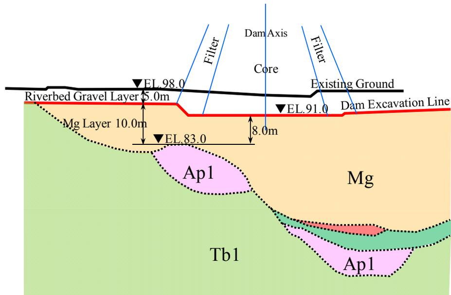
Figure 5. Considered Cross-section (No. 6+50)
