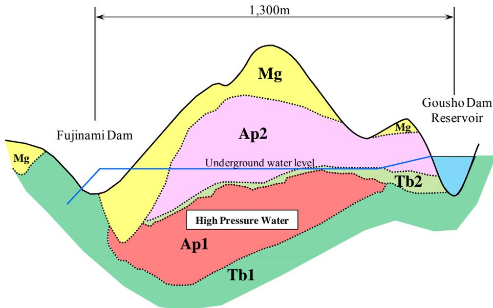
Figure 4. The model of underground structure
