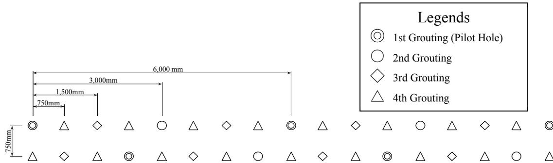
Figure 10. Ap1 Shutoff Curtain Grouting Layout
