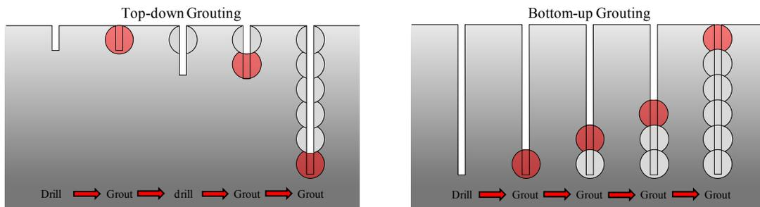
Figure 9. Grouting Method
