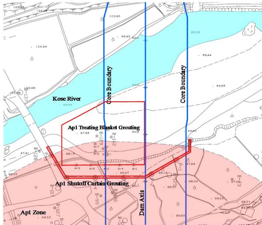
Figure 11. Ap1 Treating Blanket Grouting Plan
