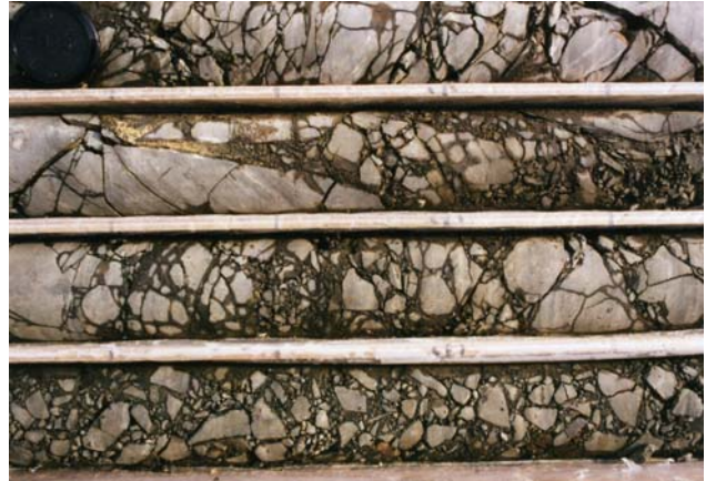
Figure 1. Boring core of Cretaceous cracky shale obtained by the highly skilled drilling engineer with traditional sampling technique of 86 mm diameter sampler
