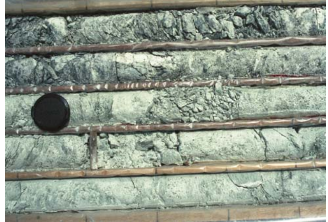
Figure 9. Boring core of Mesozoic altered chlorite schist obtained by 66 mm diameter sampler
