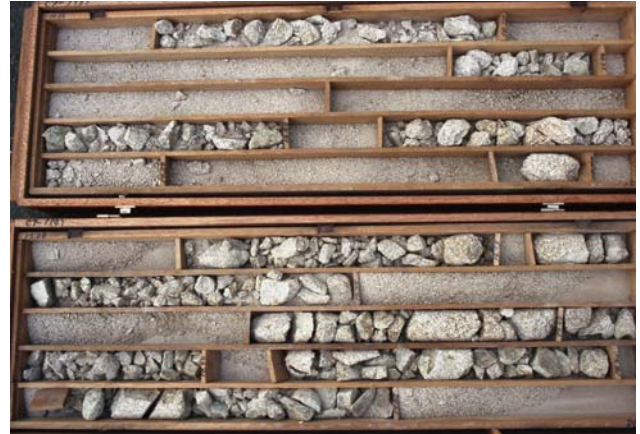
Figure 5. Boring core of Cretaceous highly weathered granite obtained by traditional sampling technique of the pre 1980's
