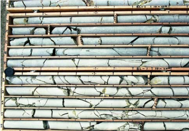
Figure 8. Boring core of Miocene cracky rhyolite obtained by rotary double-tube sampler with sleeve
