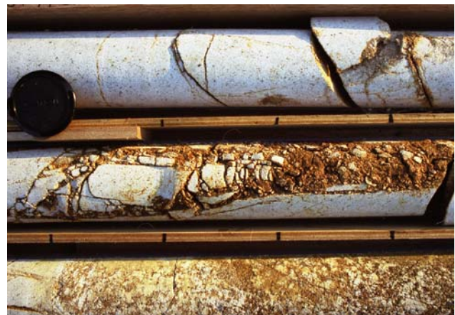
Figure 13. Boring core of Cretaceous granite obtained by high quality boring core sampling technique by use of air bubble
