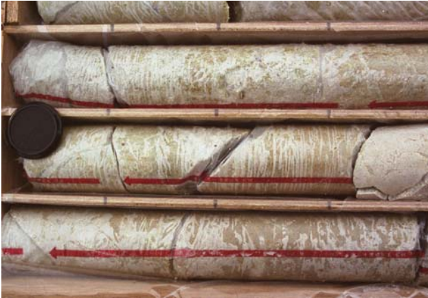
Figure 4. Boring core of Cretaceous deteriorated granite obtained by rotary double-tube sampler (86mm diameter) with sleeve
