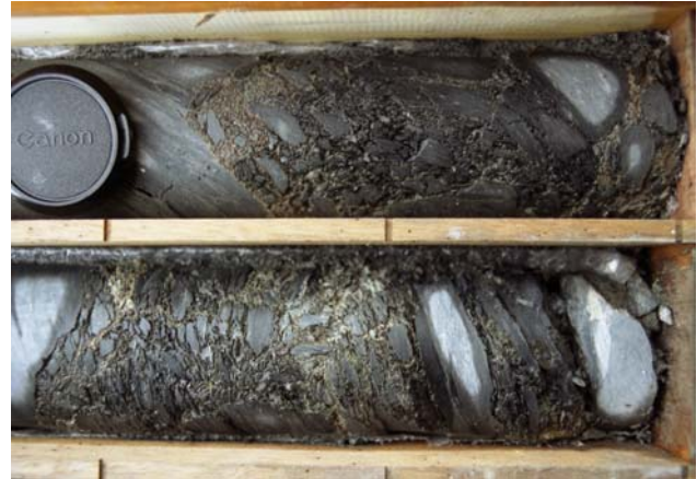
Figure 12. Boring core of fault zone of Paleozoic alternation of sandstone and shale obtained by high quality boring core sampling technique by use of water-soluble polymer solution
