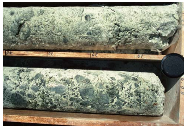
Figure 11. Boring core of Mesozoic altered chlorite schist obtained by 116 mm diameter sampler
