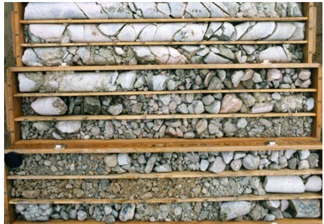
Figure 16. Boring core of Cretaceous cracky granite obtained by 86 mm diameter
