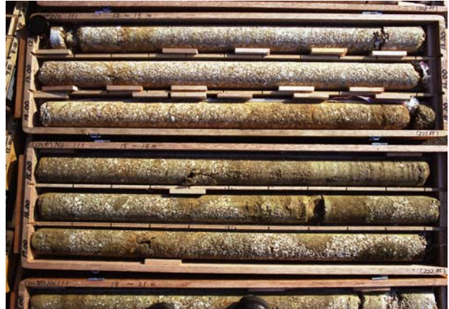
Figure 15. Boring core of Cretaceous highly weathered granite obtained by high quality boring core sampling technique of 86 mm diameter sampler by use of air bubble
