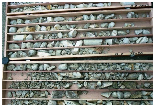
Figure 7. Boring core of Miocene cracky rhyolite obtained by traditional sampling technique of the pre 1980's
