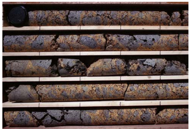
Figure 3. Boring core of Pleistocene hyaloclastite obtained by the highly skilled drilling engineer
