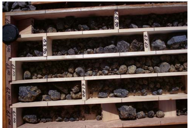
Figure 2. Boring core of Pleistocene hyaloclastite obtained by the unskilled drilling engineer
