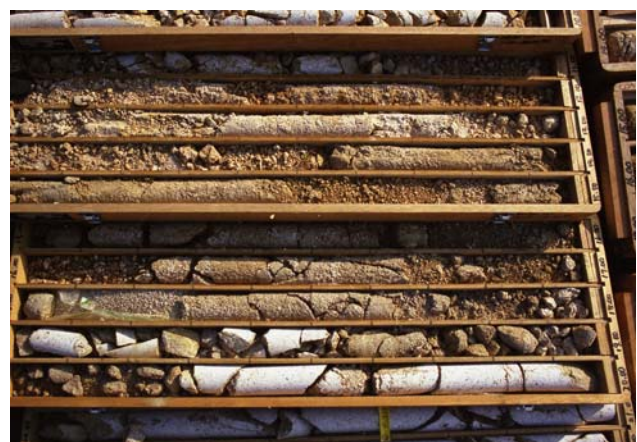
Figure 14. Boring core of Cretaceous highly weathered granite obtained by traditional sampling technique of 66 mm diameter
