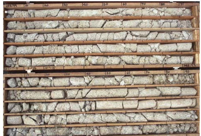
Figure 6. Boring core of Cretaceous highly weathered granite obtained by rotary double-tube sampler with sleeve
