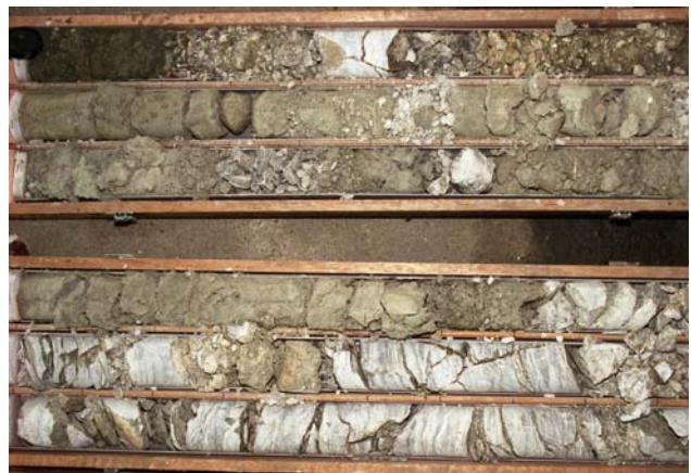
Figure 17. Boring core of fault zone of Paleozoic alternation of sandstone and shale obtained by high quality boring core sampling technique by use of air bubble
