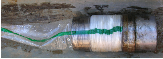
(a) Core pack tube as equipped
