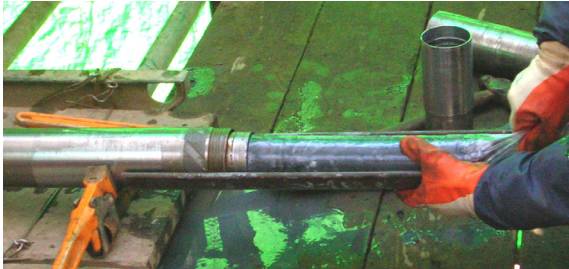
(b) Core wrapped in a core pack tube
