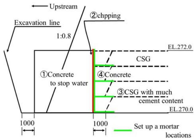
Figure 10. The outline of construction procedure near seepage control concrete: junction of the transverse direction of a dam axis
