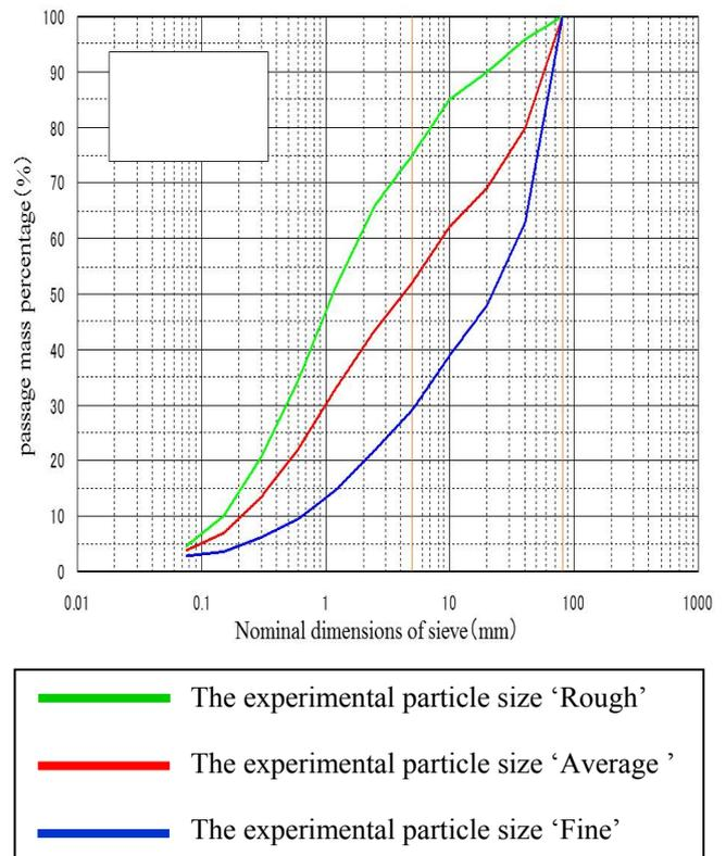
**Figure 5. Range of Grain size distribution**
