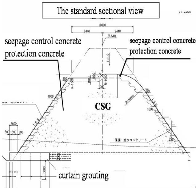
Figure 2. The standard sectional view of the Kasegawa secondary dam (overflow section)
