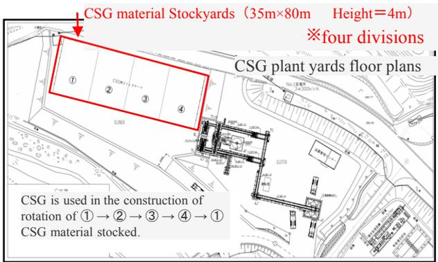
Figure 8. CSG plant yard plan view
