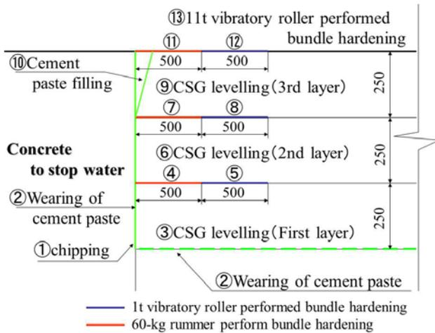
Figure 11. The outline of construction procedure near seepage control concrete: junction of the parallel direction of a dam axis
