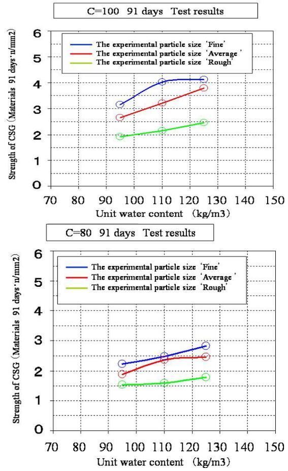
Figure 7. "Diamond" for unit cement content  $C=80\text{kg/m}^3$  and  $C=100\text{kg/m}^3$
