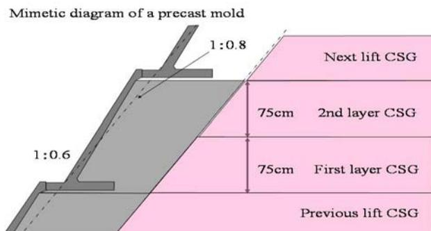
Figure 12. Schematic diagram of a precast form
