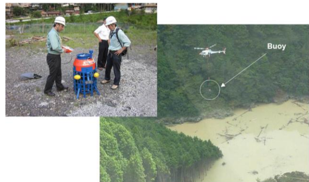
Figure 11. An aerielly-conveyable floating water level gauge
