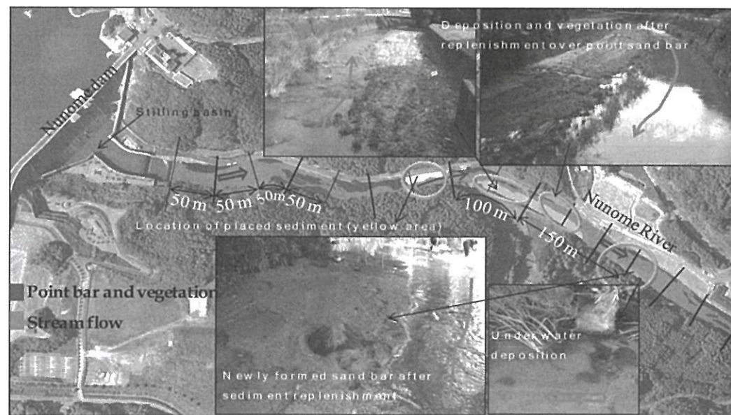
Figure 9. Aerial photographs of Nunome dam with the downstream reach of Nunome River. Morphological changes and the self forming sand bar due to sediment replenishment below the dam (14-10-2009).
