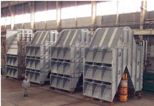
Figure 12. Temporary assembly test of all atain-less intake tubes at the manufacturing factory.
