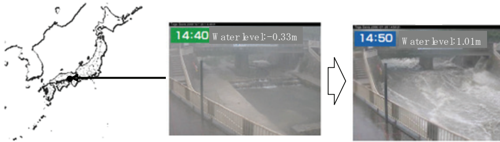
Photo. View of abrupt rise of the water on the Toga river (Kobe city in Hyogo prefecture) (Construction bureau of Kobe city)
