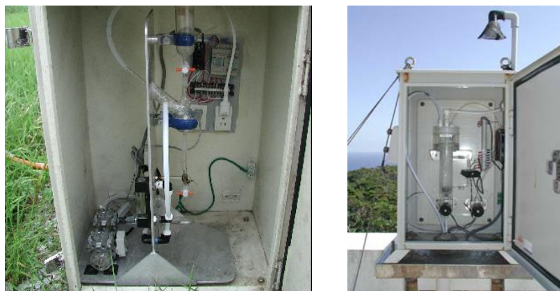
Fig. 2 Equipments for monitoring of airborne salt content
