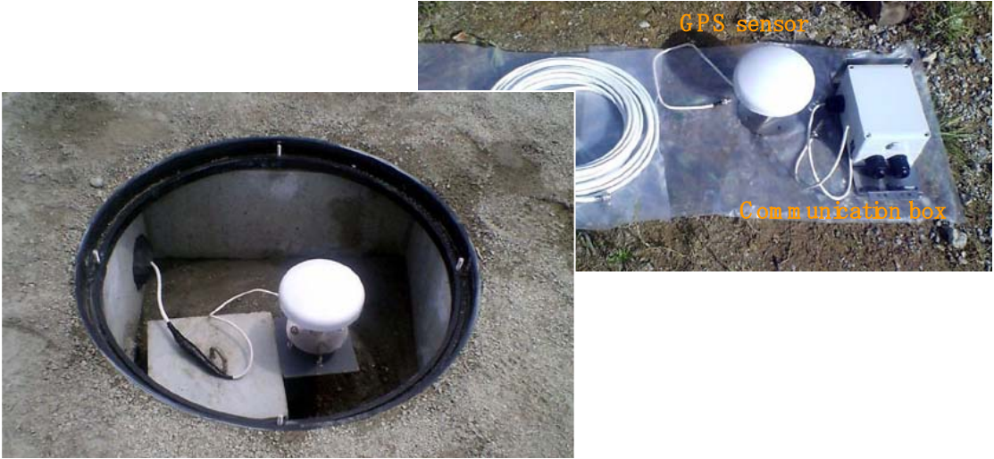
Fig.6 Backfill type GPS sensor
