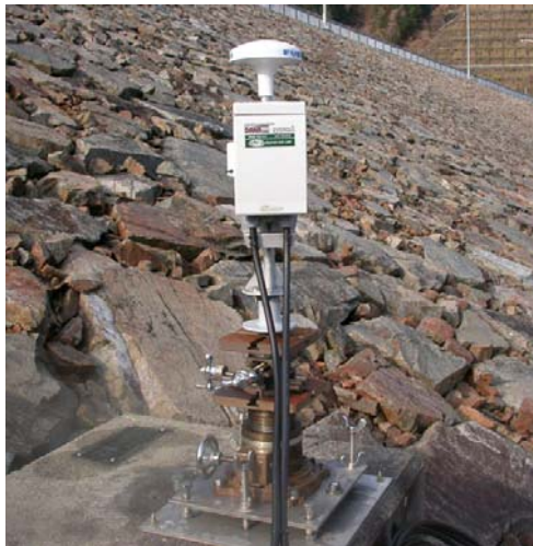
Fig. 9 GPS sensor, and comparison between numerical calculations and on-site experiment results
