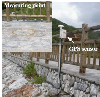
Figure 5 Installation conditions of GPS sensors
