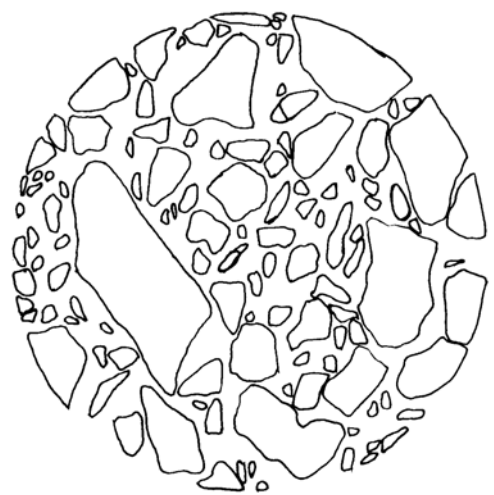
Figure 5. Image of traced boundary between aggregate and mortar.
