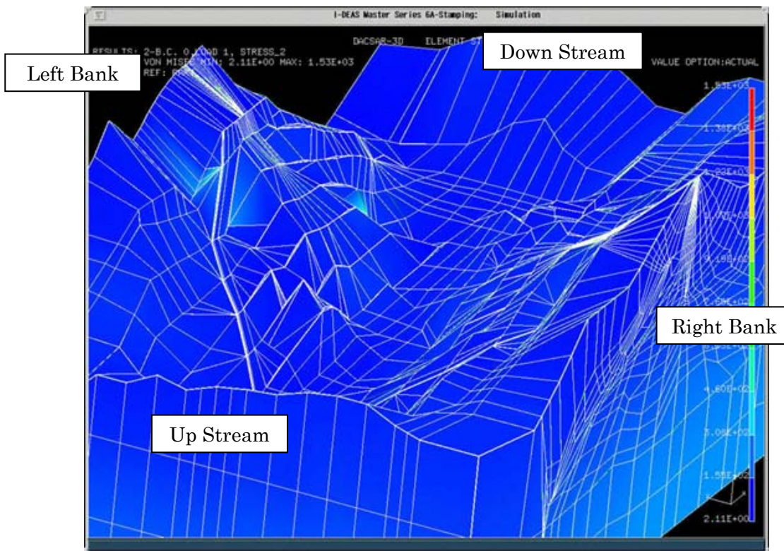
Figure.14 Foundation rock shape of Yasio Dam
