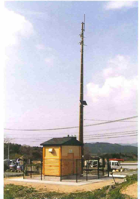
Rainfall gauging station To observe rainfall automatically, there are three stations in the upstream area of the dam and one is at Agigawa Dam Operation and Maintenance Office.
