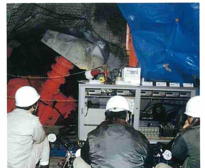
▲ In-situ shear test of cracks with low dip
