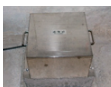
Seismograph in the base of the dam body
