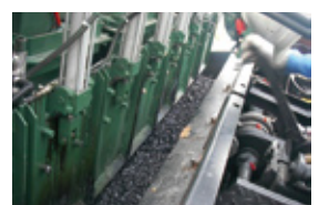
Gate type supply system
