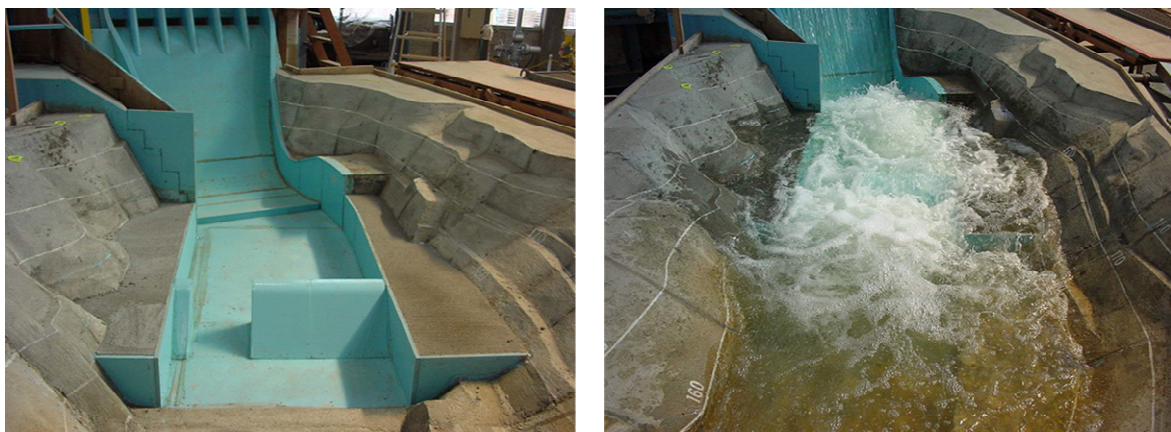
Figure 9: Flow station of hydraulic model experiment of the construction stage
