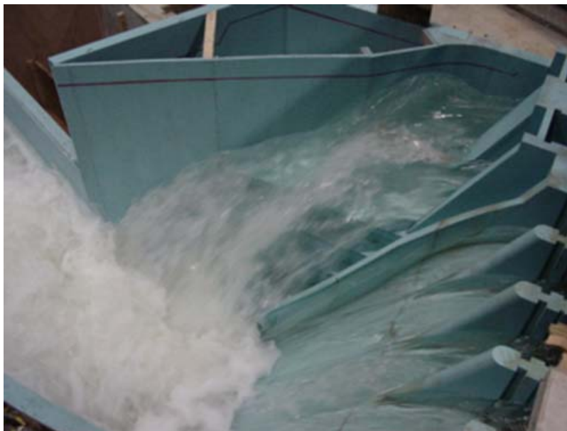
Figure 8: Flow station of hydraulic model experiment (training channel part: final design)
