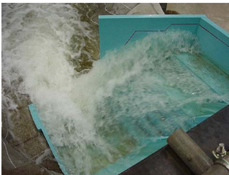
Figure 6: Flow station of hydraulic model experiment (training channel part: original design)
