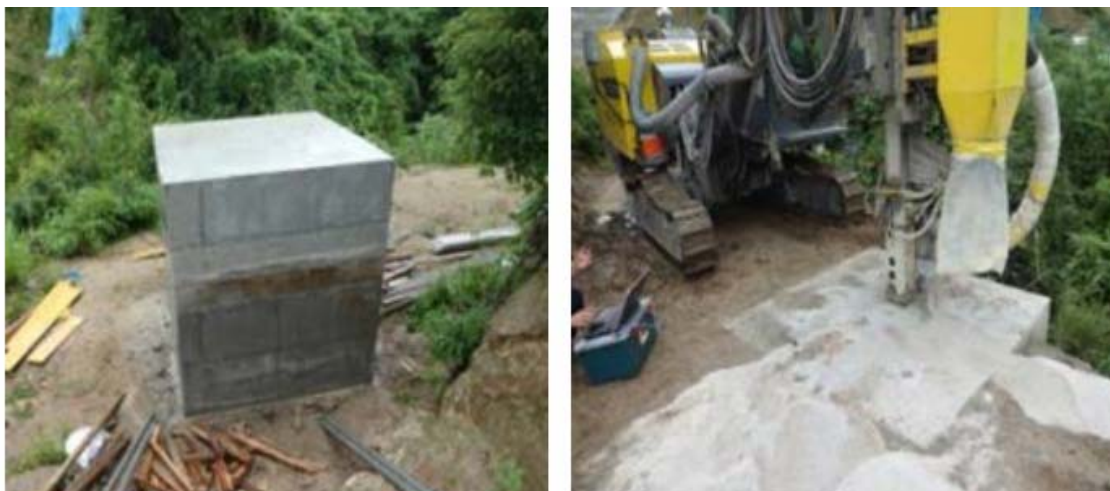
Figure 9: Experimental condition of a layered concrete block
