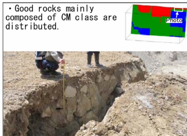
Figure 16: Verification result of the good rock area estimated by the drilling survey
