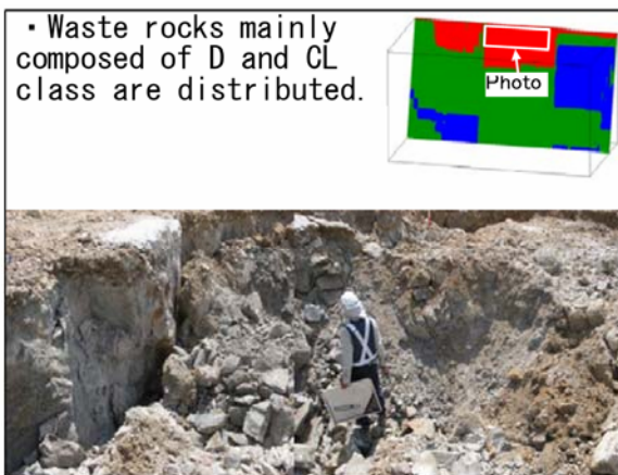
Figure 15: Verification result of the waste rock area estimated by the drilling survey
