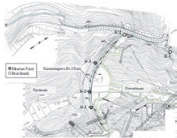
Figure 12. GPS Equipment Layout at Kuromatagawa No.2 dam
