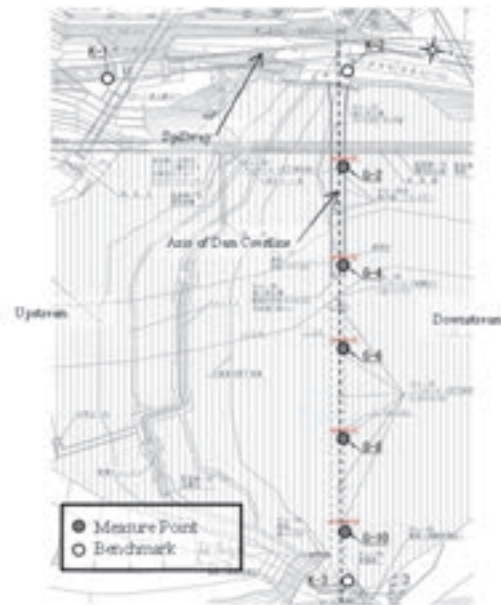
Figure 14. GPS Equipment Layout at Miboro dam
