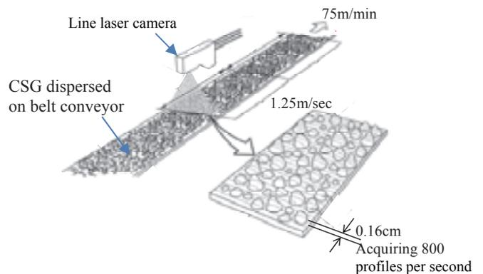
**Figure 6.** Optical cutting method using line laser camera
