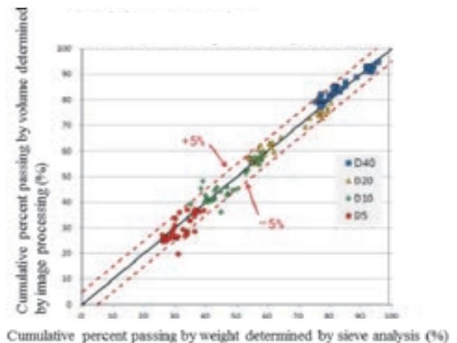
**Figure 13.** Comparison of particle size distributions: sieve analysis (weight ratio) vs. image processing (volume ratio) (Cumulative percent passing: sieve analysis vs. image processing (Cases 1 to 3))
