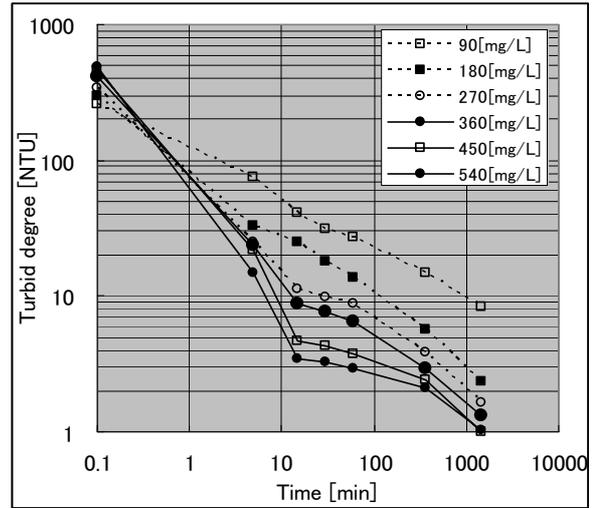
Fig. 3.1 Changes in the degree of turbidity
