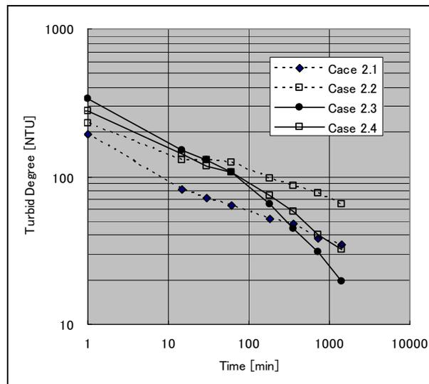
Fig. 3.3 Changes in the degree of turbidity
