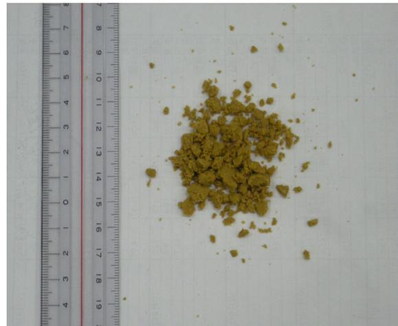
Photo 3.1 The allophane used in the experiment
