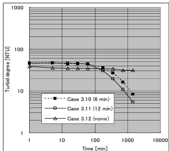
Fig. 4.4 Change in degree of turbidity (Shimokubo)(Cases 3.10, 3.11, and 3.12)
