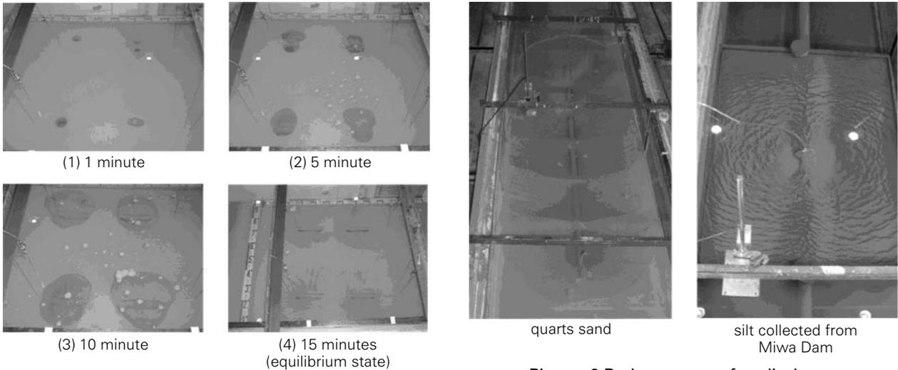
Picture-1 Geometry change of the sand bed after initiation of suction flow
