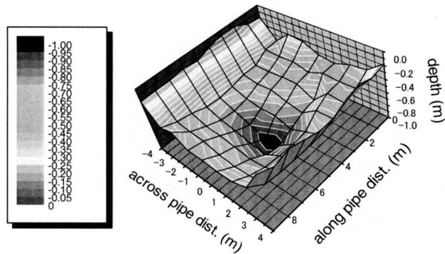
(2) Bird's-eye view of silt bed after discharge
