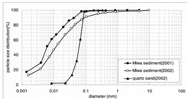
Figure-4 Diameter distributions of sediments used for the experiment
