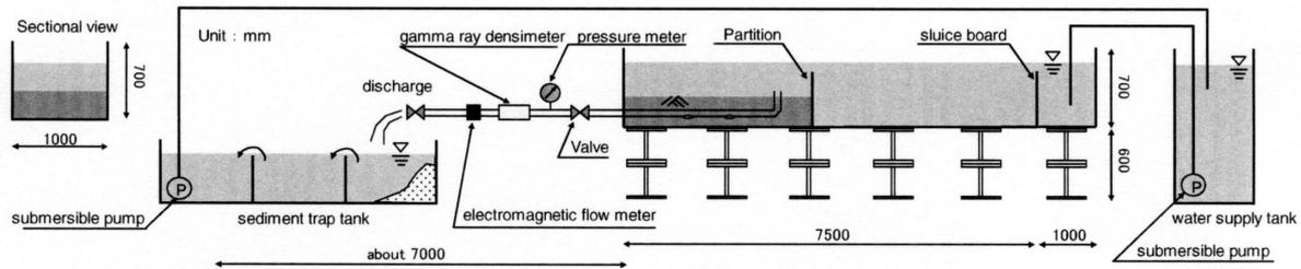
Figure-3 Cross-view of experimental facilities
